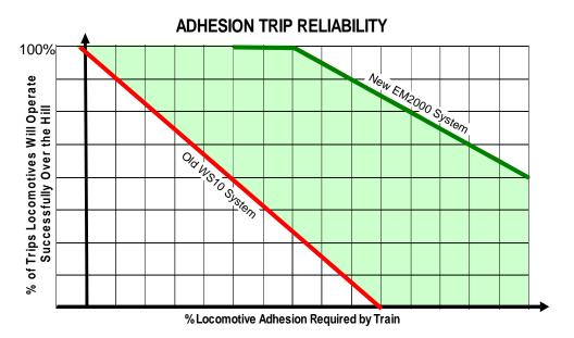
Improved adhesion and radar based wheel slip control increase trip reliability allowing for better fleet utilization. Shaded area indicates improvement over WS10.
